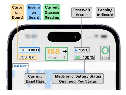
Tapping the top of the screen will bring up a History screen with information on changes implemented by the most recent loop cycle. Tapping the pump status will bring you to pump settings.
